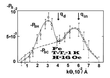
Figure 14: Crossover to dipolar critical dynamics in the chiral channels;  $\kappa$ ,  $q_d$  and  $q_{in}$  are defined in the text. Dashed line shows the prediction in the exchange approximation
