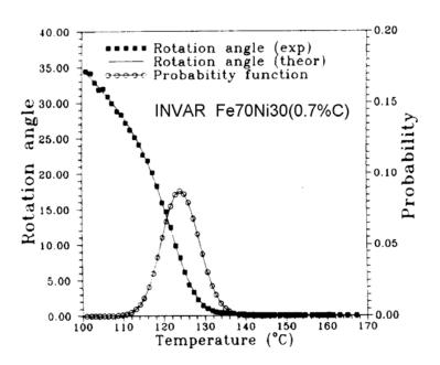
Figure 7: The temperature dependences of rotation angle of polarization vector  $\mathbf{P}$  and probability function of local  $T_c$  in invar alloy Fe<sub>70</sub>Ni<sub>30</sub> (0.7 at.% C)
