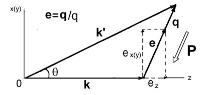
Figure 2: Scheme of small-angle polarized neutron scattering. **P** is the direction of magnetic neutron scattered polarization
