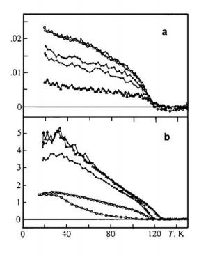
Figure 18: Temperature dependences of (a) the magnetic scattering intensity  $I_m$  with  $q = 0.01 \text{ Å}^{-1}$  and (b) the integrated magnetic scattering in the range  $q < 0.003 \text{ Å}^{-1}$  for  $\text{Sm}_{1-x}\text{Sr}_x\text{MnO}_3$  sample with x = 0.4 and H = 0 ( $\bullet$ ), 130 ( $\bigcirc$ ), 800 ( $\Box$ ), 1240 ( $\nabla$ ), 4200 Oe ( $\Delta$ ). The data for the x = 0.25 sample ( $\Box$ ) for H = 0 are shown too
