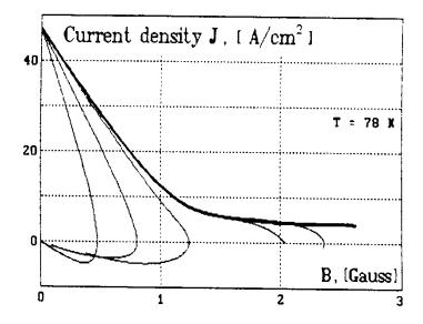
Figure 9: Internal field dependences of the current density at T = 60 K. Thick line corresponds to the distribution of B(y) at  $H \ge H_{C2}$
