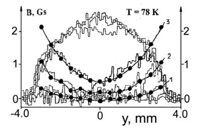
Figure 8: Visualization of magnetic flux B in Y-Ba-Cu-O ceramics with external magnetic field switched on (curves 1,2,3 for H = 2.2, 3, 1 and 4 Oe, respectively) and switched off (trapped flux) for values of H from 0.45 to 7.2 Oe
