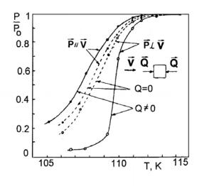
Figure 5: The dependence of P(T) in alloy Pd-Fe (4 at.%) near  $T_c$  without loading (Q = 0) and at uniaxial compression ( $Q \neq 0$ )
