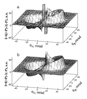
Figure 16: Spin wave antisymmetric scattering  $\Delta I$  in the detector plane for Fe<sub>50</sub>Ni<sub>22</sub>Cr<sub>10</sub>P<sub>18</sub>; a) experimental picture and b) theoretical calculation with parameters from experimental data: spin wave stiffness  $D = 52.74(5) \text{ meV} \text{ Å}^2$ , damping  $\Gamma_0(kR_c) = 25.2(5)$ , dipole constant  $\omega_0 \langle S \rangle = 50(3) \mu \text{eV}$
