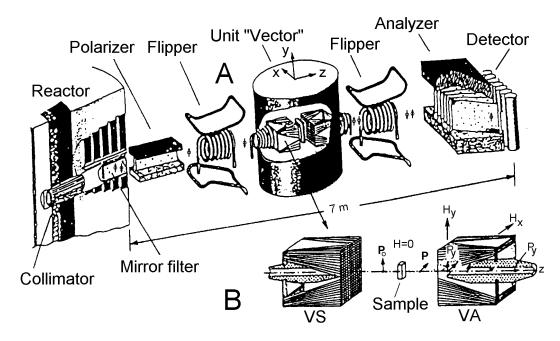
Figure 1: "A" is a block-scheme of the small-angle scattering set-up with the three-dimensional analysis of scattered neutron polarization. "B" is a unit "vector": specifying (VS) and analysing (VA) units and exmaples for measuring the  $P_y$  component of polarization are shown
