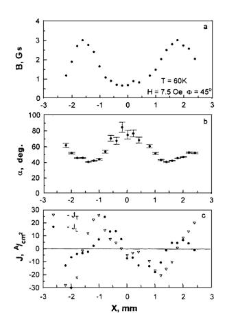
Figure 10: Sample scan for the external field rotation angle  $\phi = 45^{\circ}$ : (a) induction B; (b) angle  $\alpha$ ; (c) currents  $J_T \equiv J \perp$  and  $J_L \equiv J_{\parallel}$
