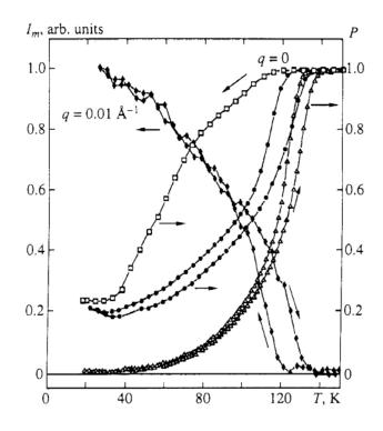
Figure 17: Temperature dependences of the polarization P in the central counter  $(q < 0.003 \text{ Å}^{-1})$  and the neutron magnetic scattering intensity  $I_m$  for and  $\text{Sm}_{1-x}\text{Sr}_x\text{MnO}_3$  sample with x = 0.4 for H = 0 ( $\bullet, \diamond$ ) and H = 4.2 kOe ( $\Delta$ ). The neutron depolarization data for the x = 0.25 sample ( $\Box$ ) for H = 0 are shown too
