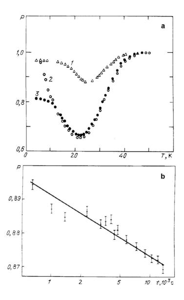
Figure 12: "a" is polarization P(T) of neutrons transmitted through the sample  $\text{Fe}_{56}\text{Ni}_{24}\text{Cr}_{20}$ : 1 is in "zero" magnetic field; 2 is in the field  $H_x = 62$  Oe after preliminary cooling to 4.2 K in zero field; 3 is measuring in the field  $H_x = 62$  Oe. "b" is the long-time logarithmic relaxation from state 2 to state 3 (curves in "a") at T = 8 K:  $P(t) = P_2 - S \ln(t/t_0)$ , where S is a coefficient of consequence
